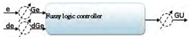
Fig. 9. Structure of a fuzzy logic controller. Ge, dGe and Gu are the adaptation parameters of fuzzy controller.
